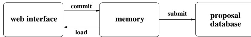
Figure 3: Illustration of the concept of an intermediate memory area for proposal information storage that has not yet been submitted into the proposal database.
